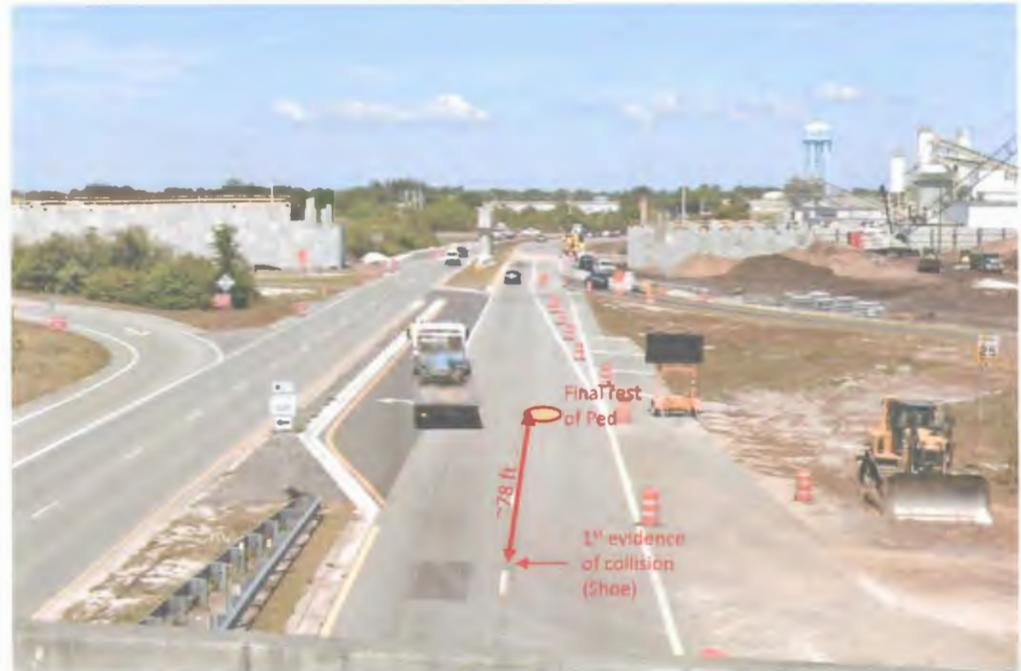
Layout of evidence (from 3D laser scan data)
